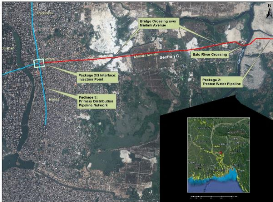
Figure 4-4: P2 Pipeline Route up to Injection Point
